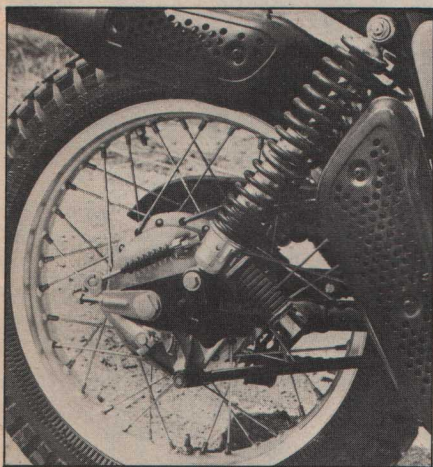
(LEFT) Rear shocks are straight from the stone age. Muffler is quiet, but quite heavy. (RIGHT) The front forks boast of over seven inches of travel. Brakes, front and rear, were surprisingly good.
