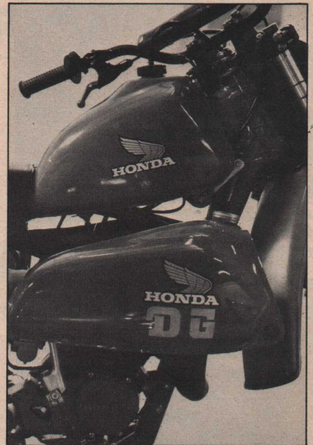
DG's plastic "Works" tank will be similar to tank at top but will have the stock mounting points of the stocker (bottom).
