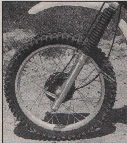
Front forks deliver just over nine inches of travel, and are surprisingly plush for a budget bike.
