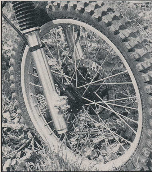
Speedo and front brake setup is well designed and well protected. Disc brake is the best enduro stopper we've ever used.
