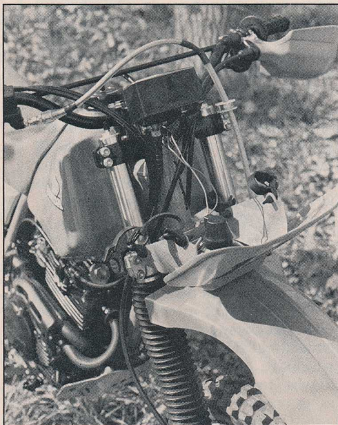
The front of the bike is very uncluttered, a refreshing change on the XR's. Headlight/numberplate weighs mere ounces, and can be fitted with a quartz halogen bulb.
