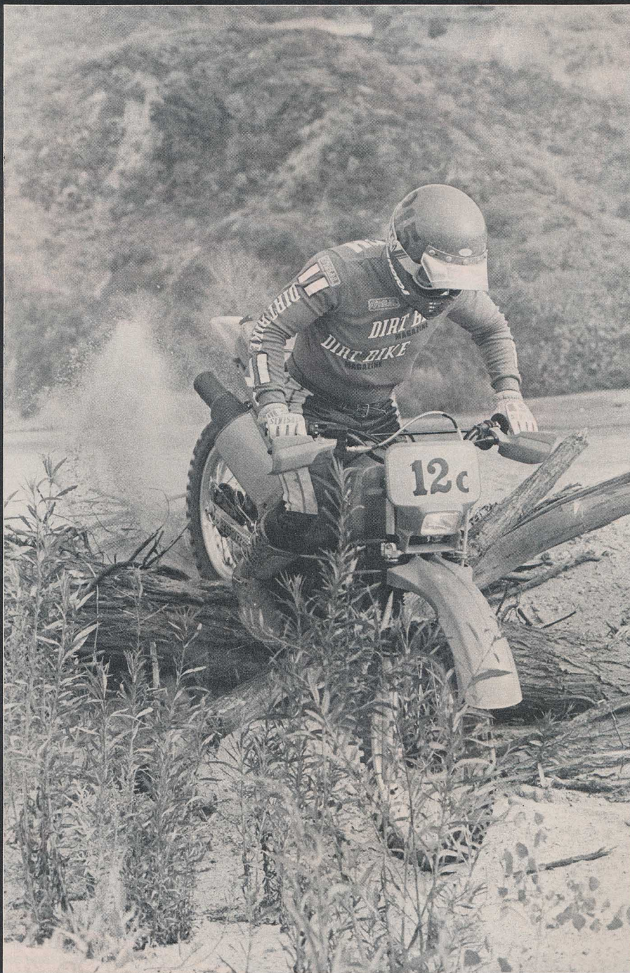
A wide spread of power makes the XR a fun bike to poke around on. Short wheelbase is nice in tight stuff, but nasty at high speeds.
