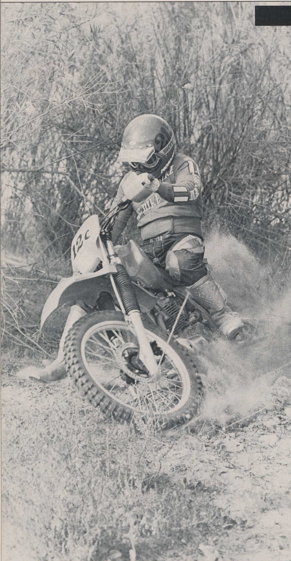
Soft rear suspension was primary cause of front-end washout. A stiffer rear spring should be the XR owner's first purchase.
