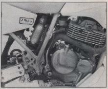
Oversized fins are the only obvious indication that all is not stock inside the Barnum DR385. The header pipe is designed to accommodate the piggyback RM shock, should you decide to spring for one.
