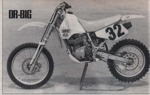
more rear-wheel travel, along with more consistent damping. Barnum modified the steering stem on a set of '90 RM250 triple-clamps and bolted the complete fork assembly on the Antunez DR385. He also went to a three-tooth-larger rear sprocket (a 51T) to provide more grunt out of corners.
