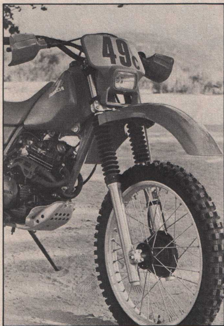
The 36mm Kayaba forks are skinny compared with the tubes found on the XR's two-stroke competition, but they work fine for trailriding.
