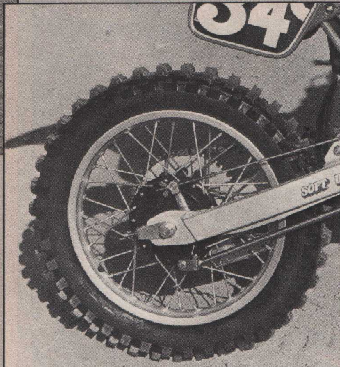
A floating rear brake is average and goes away quickly at any hint of moisture. The aluminum swingarm looks stout, but we've heard rumors of breakage problems. Ours never gave us any grief.
