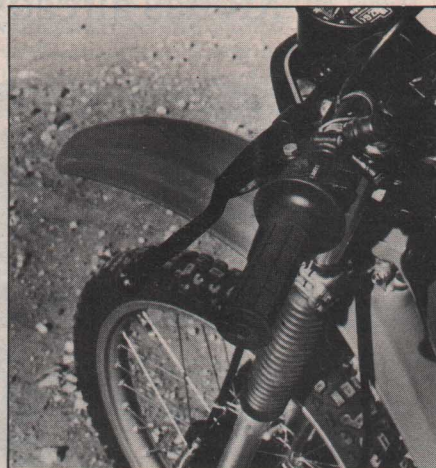
Levers are of a dog-leg design, with reversed ball ends to lessen brush-snagging.
