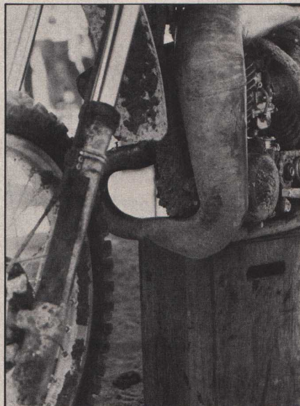
At the halfway point in the first moto Lackey's Yamaha slowed considerably. A smashed header pipe was the culprit.
