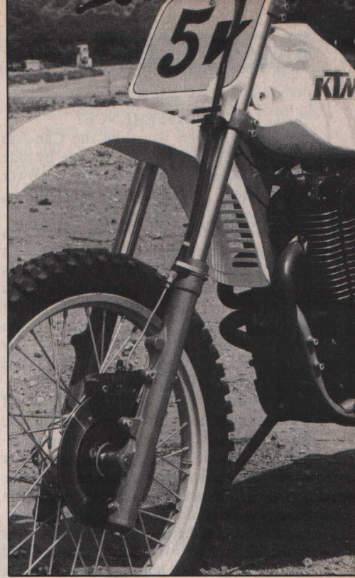
A sanitary Brembo disc brake is attached to the finest set of Marzocchi forks we've ever used.
