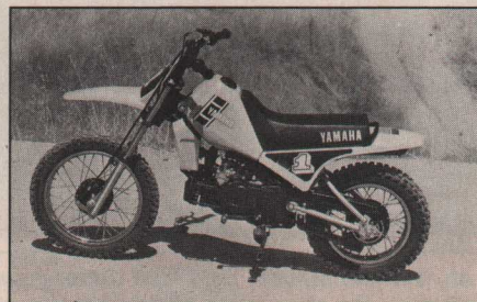
Yamaha PW80: a small, light three-speed automatic.
