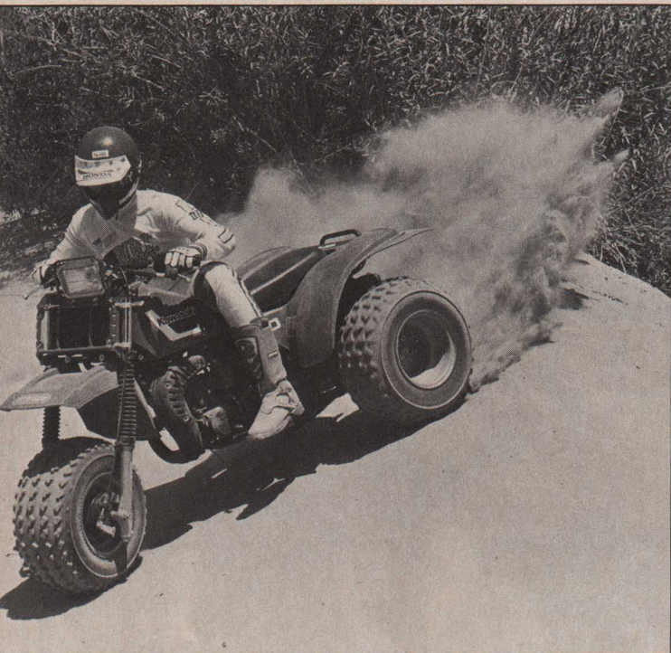
The KXT is a very stable slider, due mostly to the firm-walled low-profile tires and 10-inch wheels.
