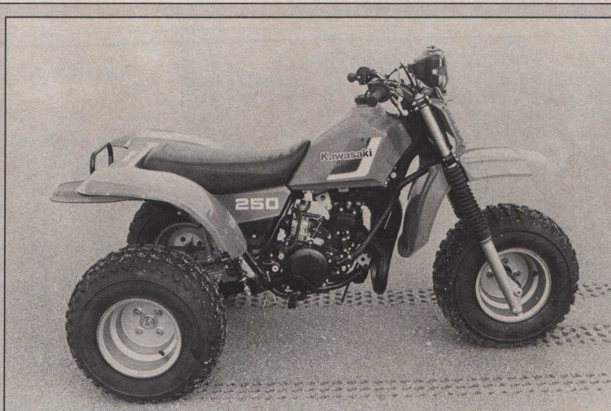
Single-strut Uni-Trak is a dead ringer for the motorcycle version. Rebound damping is adjustable.
