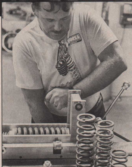
Gil checks the rate in his spring tester and finds that his math was right on the button.
