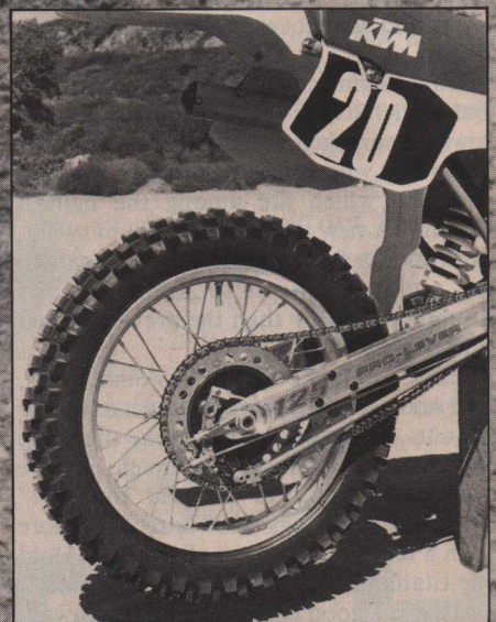
New slim aluminum swingarm cradles a double-leading shoe rear brake setup taken directly from the 1983 250LC.
