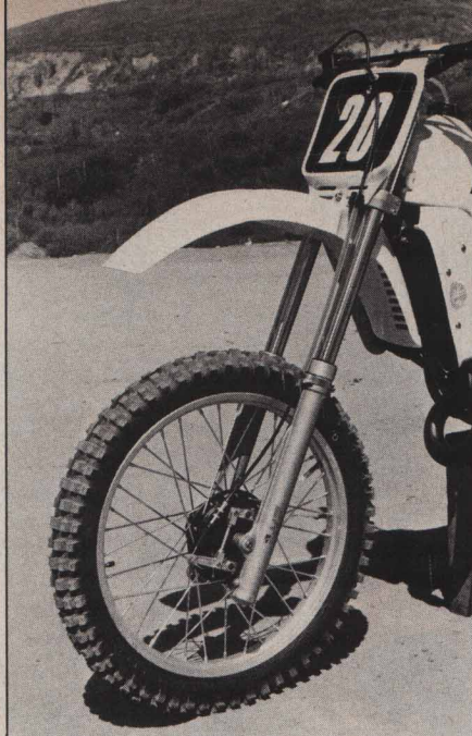
The 40mm forks (Marzocchi) are the same as those found on the 250 bikes.
