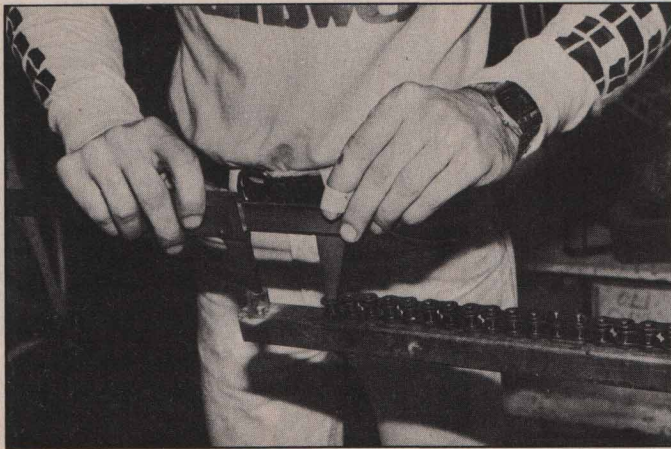
Measuring stretch was easy. The tested chain was slipped over a pin and compared with the original length.
