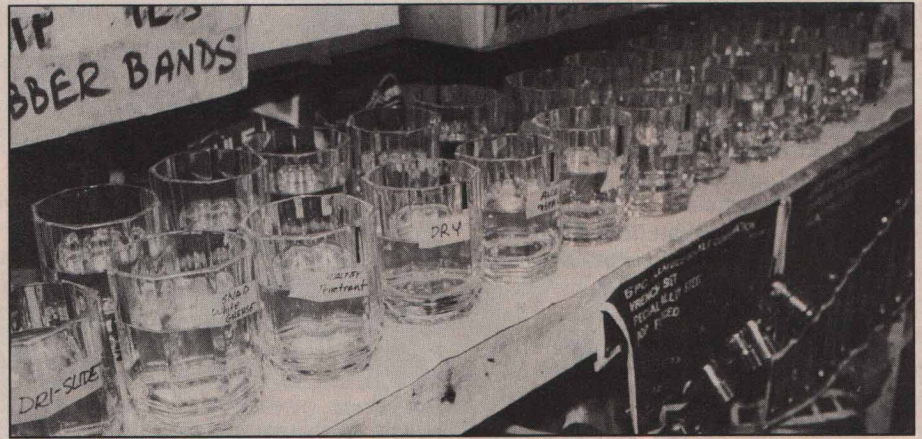
For the corrosion test, we simply coated links with a lube, dropped them in a glass of tap water, then sat back and observed the rust... or lack thereof.
