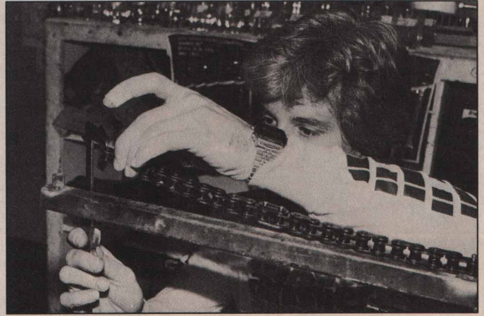
To test wear, we put the chain over a welded pin, then measured the total side deflection.
