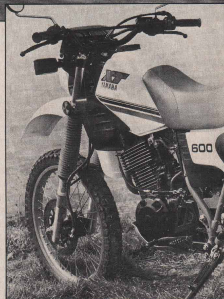
Folding levers, a skid plate and the motocross-bred safety saddle are nice touches for the dirt oriented. The tachometer, air scoops and plush suspension are for the street minded.
