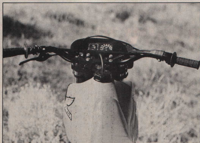
The tank is large, but not cumbersome. There's a natural flow from the seat onto the tank. Bars are too wide for tight woods; hack an inch off each side.
