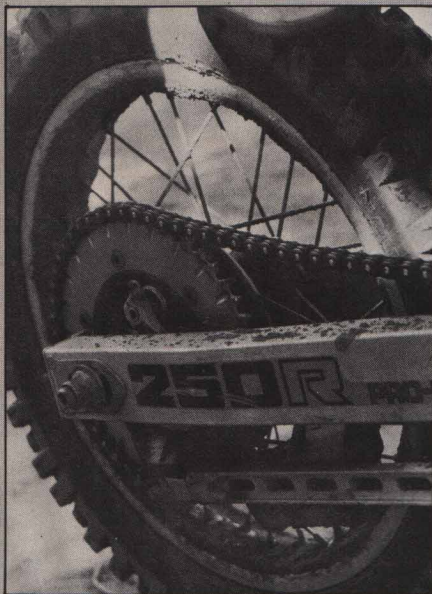
All of the stock CR sprockets wear out quickly. We opted for a Sidewinder unit that's a little heavier, but lasts far longer.
