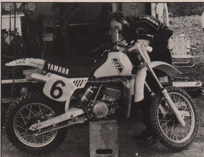
All of the works Yamahas are fitted with a new linkage that resembles something in between the Honda and the KTM. Ohlins handles the rear damping chores and the 500 is Power Valved.
