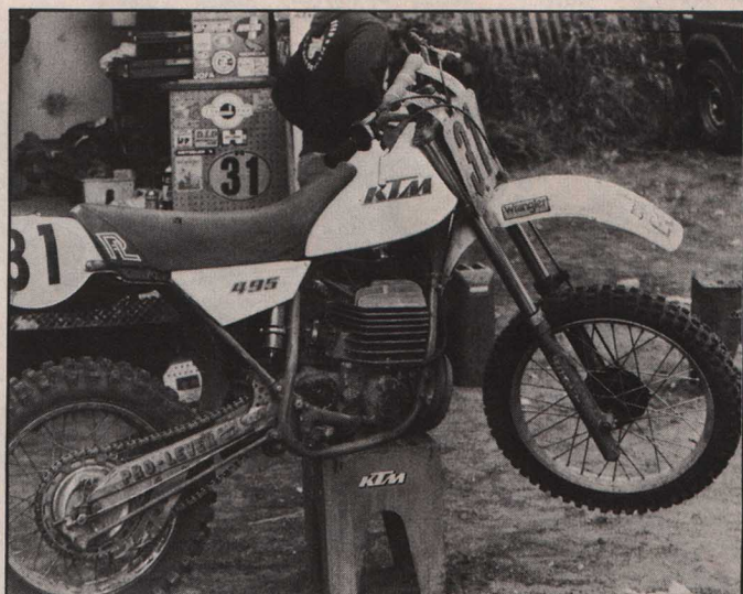
John Finkeldey's 495 KTM has had very little done to it as far as the motor goes. The entire front end is off of a 250 water-cooler, as is the front wheel. This alone saves about seven pounds.
