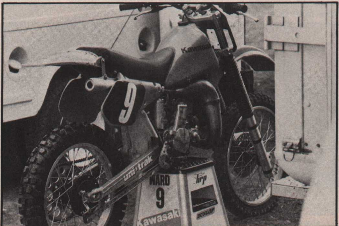
Ward's Kawa 125 is the fastest in the class. The bike sits right on the weight limit, and has the motor of death. Muffler is stock; both the swingarm and the linkage are hand-machined trick-o's. □
