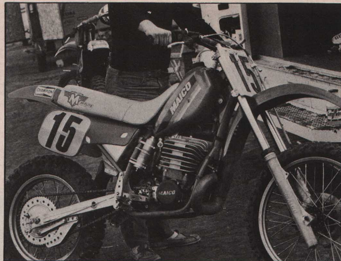
Chuck Sun's Maico is a one-off model, built just before the start of the season. Notice the lowered aluminum gas tank, Kawa front wheel and aluminum airbox. The entire chassis is lower and slimmer and the pipe goes up the left side instead of the right, like the stockers.
