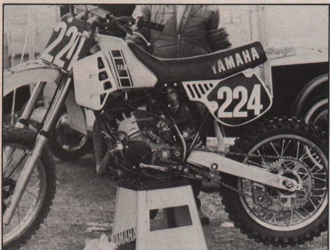
Yamaha has seen fit to focus a major amount of attention on its 125. Lechien's bike has a rotary-valve-type engine. The valve is driven off the crankshaft up to a normally placed carb. His bike is very, very fast.
