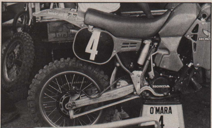
Honda's 125 runs disc brakes both front and rear. The tank is similar to the 250's design and the power is down compared with the Kawa's 125. That little bottle up by the shock reservoir is the master cylinder for the rear brake.
