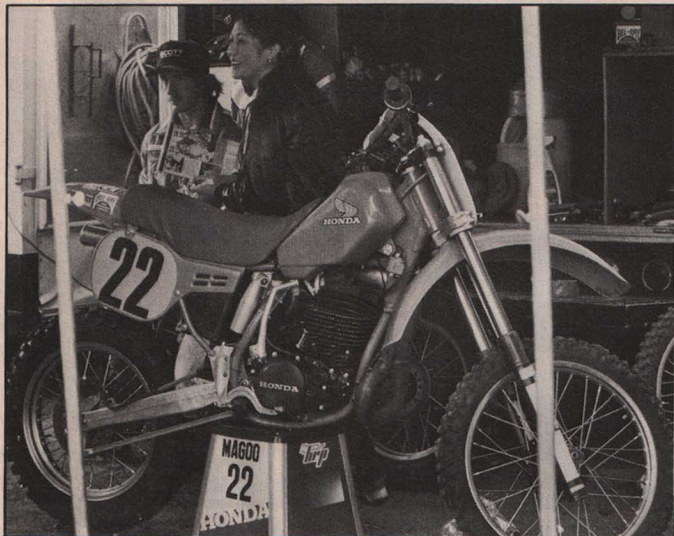
Magoo's Open Honda is fitted with the same cases that the European water-cooled versions have, only it's still air-cooled. The clutch is hydraulic rather than cable operated, and the pull is easier than on the 125s.
