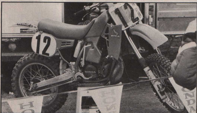
Hannah's Honda is the only red machine not fitted with a disc brake somewhere. The shock is a piggyback Showa that has adjustable compression and rebound damping. Seventy percent of the bike's fuel is carried in the lower portion of the oddly shaped tank.
