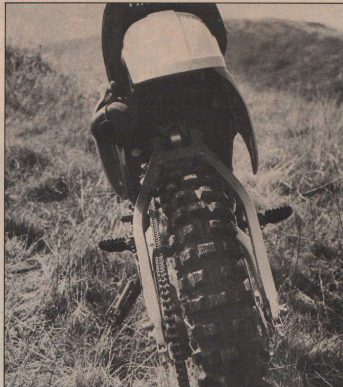
YZ125F is very slim, due to no shocks mounted on the side. There's plenty of room for increased rear end travel. Swingarm is excellent, chain and tire marginal.
