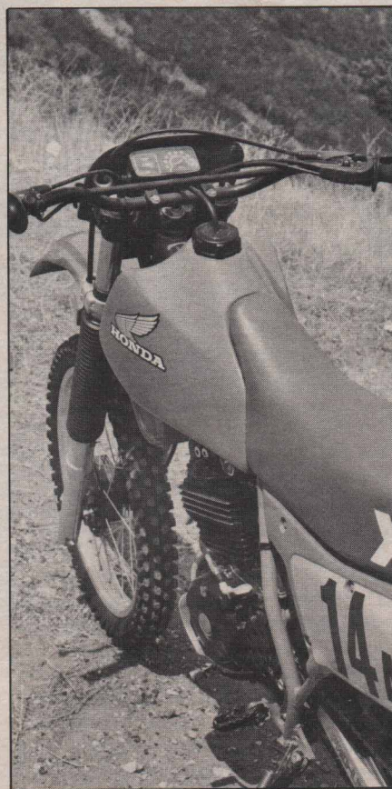
Seat/tank combo is blended perfectly—there's no way to get snagged on this bike. XR's use full speedometer rather than odometer only.
