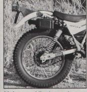
It's been a while since we've tested anything with two shocks. The rear wheel's 5.9 inches of movement is adequate for casual trailriding and off-road boulder plonking. Footpegs are high and to the rear of the traditional placement. The small saddle gets uncomfortable on long trips, but is okay for short jaunts.
