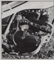
Reliability and economy are two key Reflex traits. The 195cc four-stroke powerplant sips petrol, and its time-proven design is virtually bulletproof. Kick starting is made easy by an automatic compression release.
