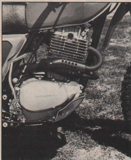
Cleanly styled engine has minimum of snaggers around cases. Small twin pipes are carefully tucked away from rider. Long kickstart lever also operates automatic compression release for easier starting. It works.
