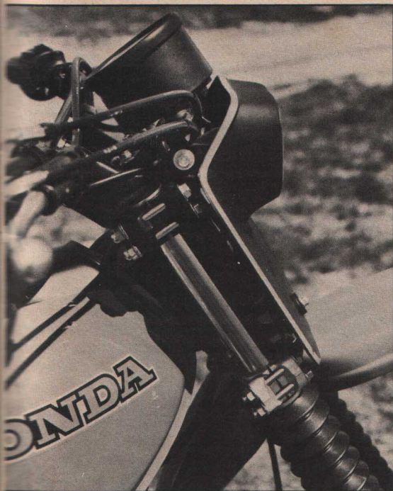
Headlight/number plate design makes sense—there is room for the speedo, and cable routing is more natural. Beefy triple clamps seem quite strong.
