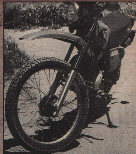
Forks actually have 7.9 inches of travel, could be a little stiffer for the dirt. Front brake is good.
