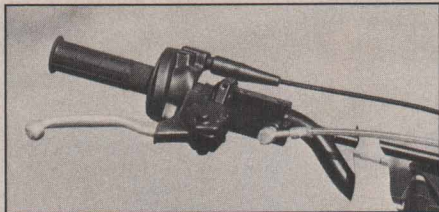
Hydraulic master cylinder is reasonably compact and resists abuse well. We managed to bend the lever, but never scratched the reservoir.
