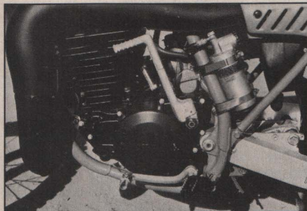
Now a five-speed, the Honda is versatile because of the torquey motor and the new gearbox. The shock features both adjustable compression and rebound damping.
