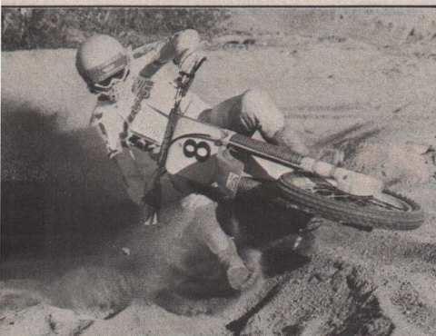
A sharp rake (26 degrees) makes for a quick handler. Slamming into a berm at speed requires a properly timed blast of throttle to keep you from plowing under.
