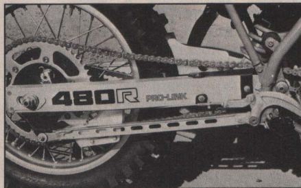
Watch the rear sprocket, it wears quickly. All of the running gear is very factory looking. The rear brake adjusts at the end of the cable, near the pedal. Loosen the jam nut and then dial in the amount of play you want in the brakes.
