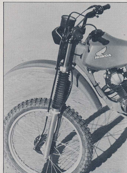
Front forks will still flex some when pushed but still work much better than last year's model. The XR's swingarm is painted chrome moly and will stand up to a lot of abuse. Tire is too small for marginal traction conditions.
