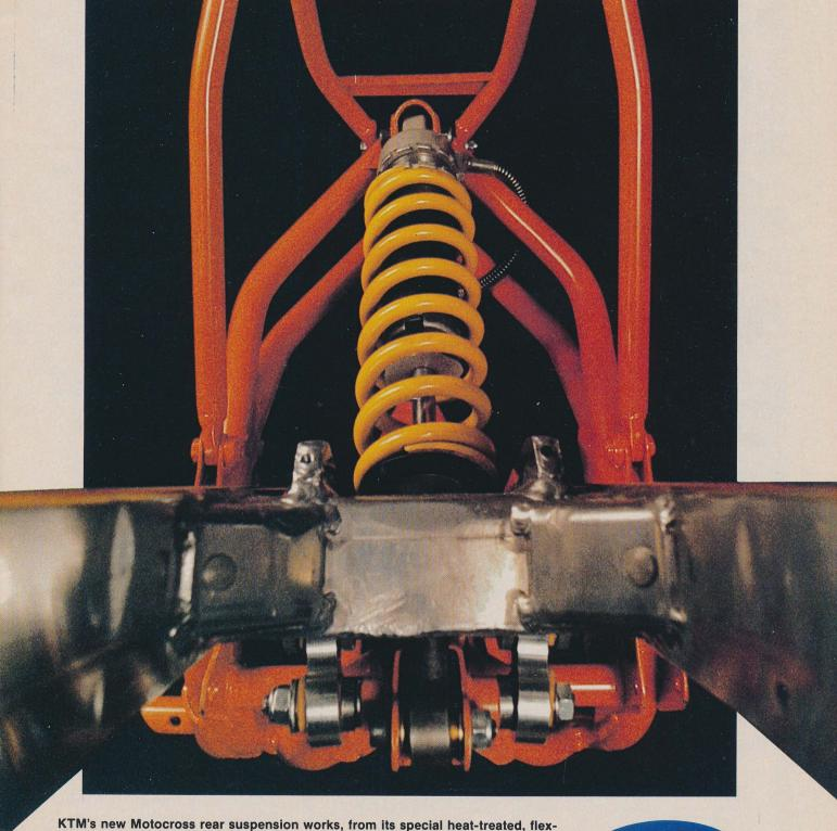
KTM's new Motocross rear suspension works, from its special heat-treated, flexfree extruded aluminum swing arm to its straight forward lever-link shock system. The reason is simple. KTM engineers evaluated all the single-shock solutions,
