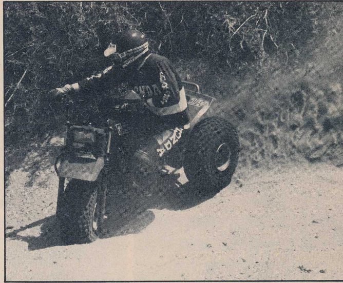
In a high-speed turn, the weighting is reversed—centrifugal force makes this ATV want to stand up on the outside wheels. Body English and a wide-open throttle keep it from doing flips.
