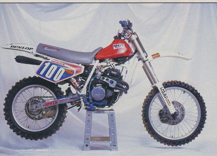
An '84 XL350. Doesn't look very much like an '84 XL, does it? George Smith, 100s rider, and White Bros., the source of most of the non-Honda items on the bike, obviously have more serious plans for the machine than Honda ever did. The White Bros. White Power suspension, at $1700, is costly but effective.
