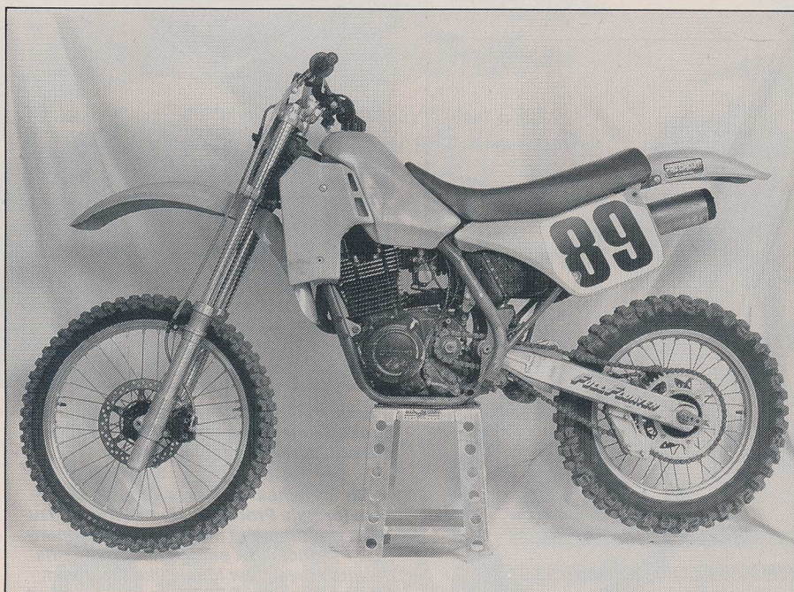
How sano was it? DC Fabrication's DRM500 was so sano it was scary. It's all Suzuki: '83 DR500 engine, '87 RM250 frame. If Suzuki started pumping these out tomorrow, we wouldn't complain.
