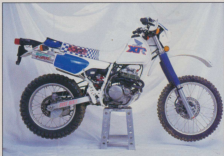
In love? DIRT BIKE's XR250L grew up, with help from XRs Only. The extended-fin 280 top end and revalved and resprung suspension might just make this 280 a better 350-class dual-sport than a certain other popular 350 dual-sport. Stay tuned for the tell-all test of both bikes.
