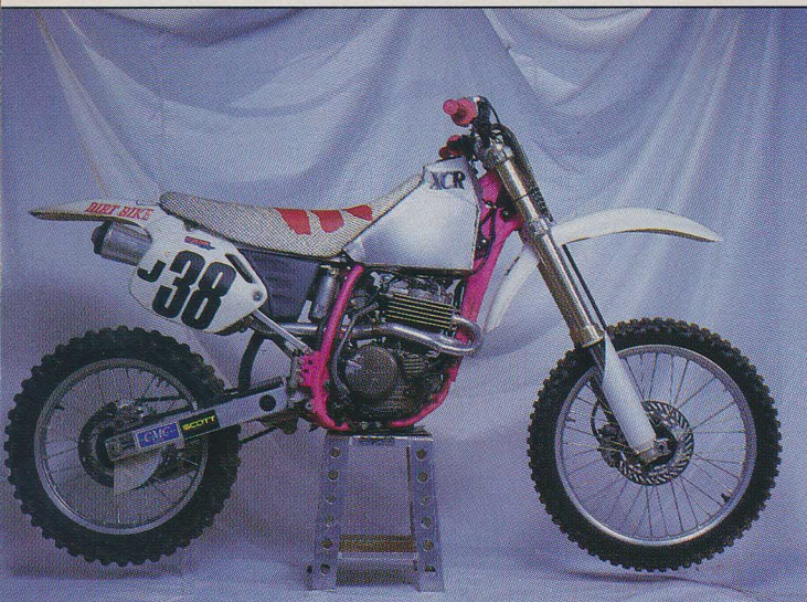
Joe Martin's XCR is the most modern CR/XR hybrid. The CR's ultra-thin tail with its jumbo airbox joins Martin's handmade tank with its flush filler cap for a smoother and slimmer-than-CR layout.
