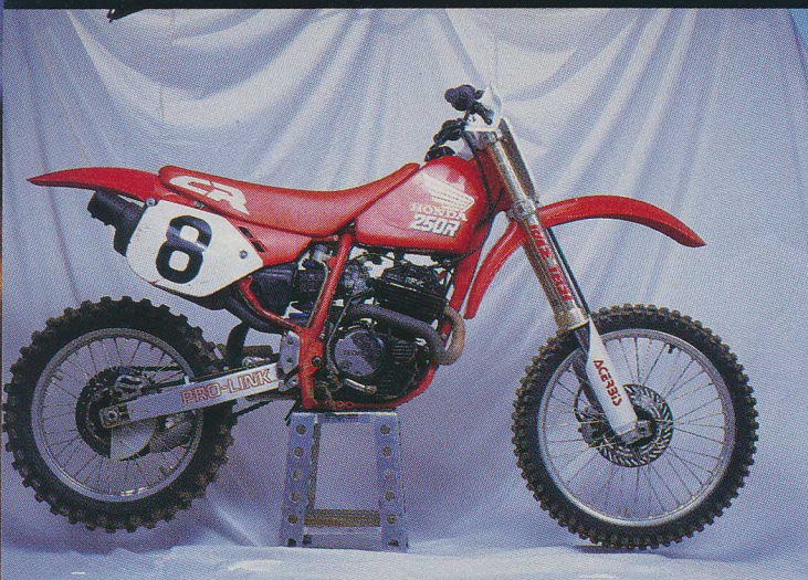
Doug Johns' CXR250 uses a heavily modified XR250 engine to propel an '89 CR125 chassis. This 228-lb. thing of beauty accelerates like an Open-class bike.
