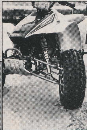
Eight inches of front-end travel allow the FourTrax to tackle the off-road world with a will. The engineers at the red factory designed this machine so it does not bump steer. In other words, when the FourTrax is pitched into a slide and the rider comes upon a bump or whoop in the middle of that slide, the Honda will absorb the bump rather than deflect as the Suzuki does.
