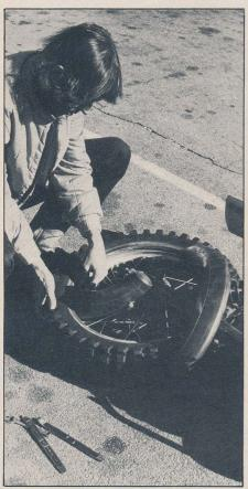
Wheel can be rotated to make installation easier. Pop the bead back on. Take the final bite where the two tube ends don't quite meet to eliminate any risk of pinching the tube. Time's up.
