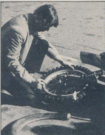
Notice the brake arm being used as an extra hand to help break the bead. Start from the valve stem and work out. Knife will be used to cut the old tube.
