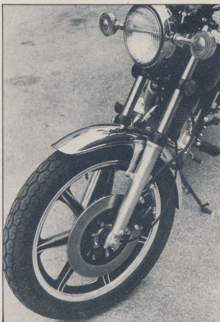
The disc brakes and cast aluminum wheels are welcome updates for the thumper.
