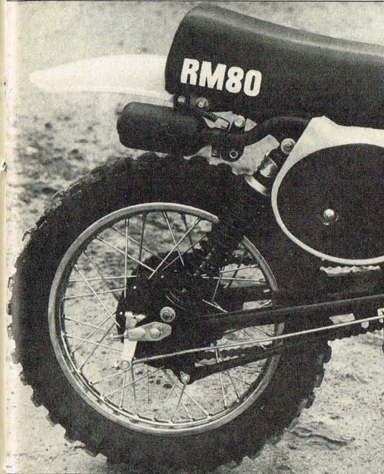
Gas shocks are new. Rear wheel travel is just under five inches.
