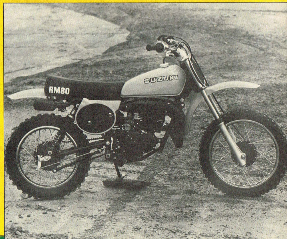
Factory porting, more compression, a six-speed tranny and a carburetor increase to 28mm highlight the engine changes.
