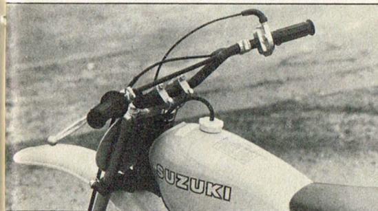
New handlebar setback allows forks to be serviced easier as well as permitting fine-tuning of the steering geometry.
