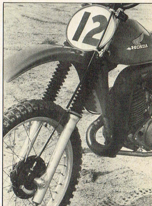
Showa magic forks. Take our word for it. They make the bumps disappear. Very works-like down to the plastic cable clamp.
