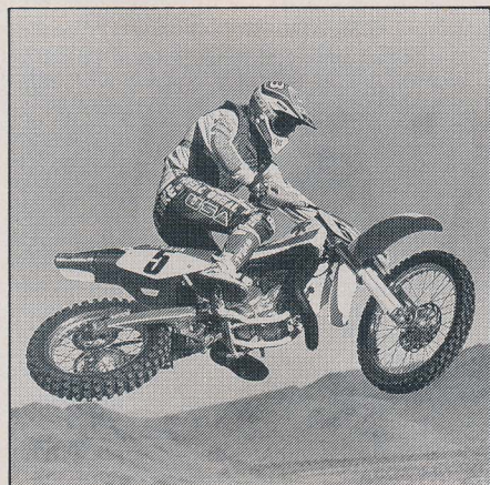
Yamaha's new WR500 isn't really a wide-ratio. It has the same gearbox as the latest YZ490, but with taller overall gearing. The 500 is so flickable we think "WR" stands for "Wild Ride."
