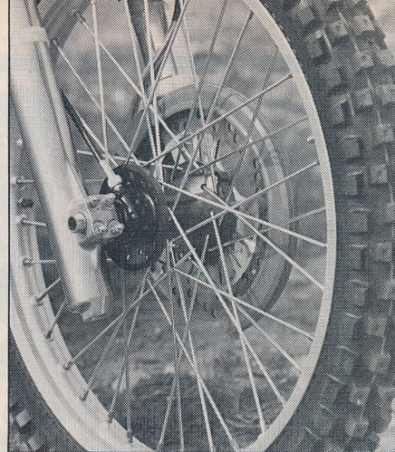
The eye-watering top-end muscle is easily harnessed by the power of the disc front brake. The fancy plastic guard, though not capable of preventing serious rock damage, should be able to keep the smaller branches from disrupting stopping ability.
