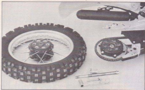
All new rear wheel can be removed in under 15 sec. The procedure requires the removal of the axle and one spacer. Axle adjusters and sprocket stay in place and go untouched. Suzuki six-day tool is all that is needed for wheel removal.
