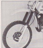
Front brake is strong and has an external return spring to prevent sticking when operated in mud. Forks are shortened RM units.
