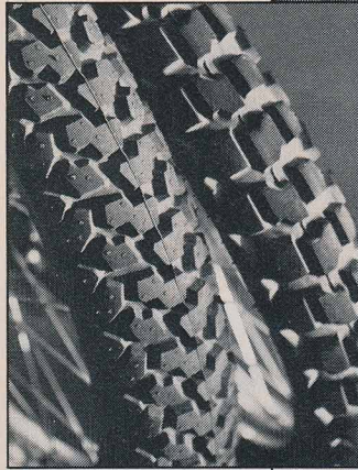
Semi-knobby stock tire (right) worked well in the dirt but gave a heavy feel during low-speed street work. A closer-patterned tread (left) cleared up the heaviness but didn't work nearly as well off-road.
