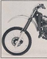
KYB-built front fork has 43mm stanchions, 11.8 inches of travel and adjustable compressiondamping blow-off valves.
