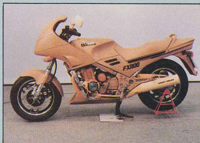
A wooden-engined, clay mock-up of the final design bears the name "FX1100." The "FJ" designation wasn't decided upon until fall of 1983.
