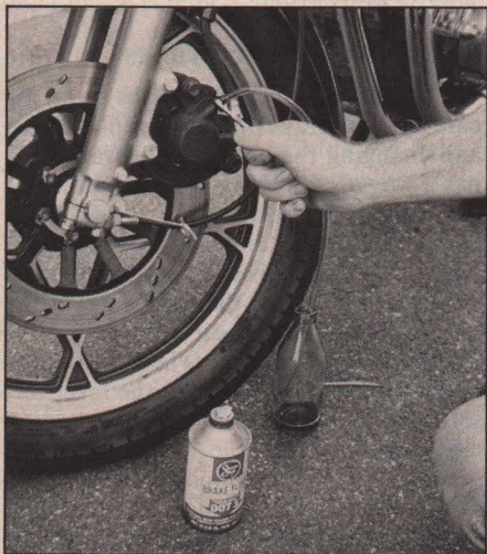
Disc brakes should be bled occasionally to clean moisture and dirt out of the hydraulic system. Keep bleeder tube higher than the bleed screw to prevent air from bubbling into the caliper.
