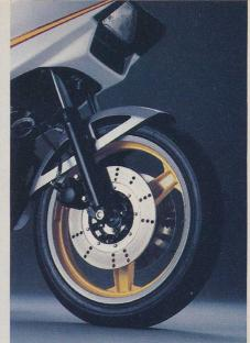
Standard calipers with the addition of Ferodo pads take care of stopping the motorcycle. Magnesium Dymag wheels, WM4 front, WM5 rear, carry Michelin tires, an S 41 (PZ 2 compound) in front and a M 48 at the rear.
