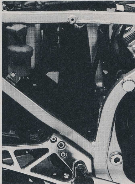
The single air-adjustable shock mounts vertically in the frame. Rebound damping is four-way adjustable.
