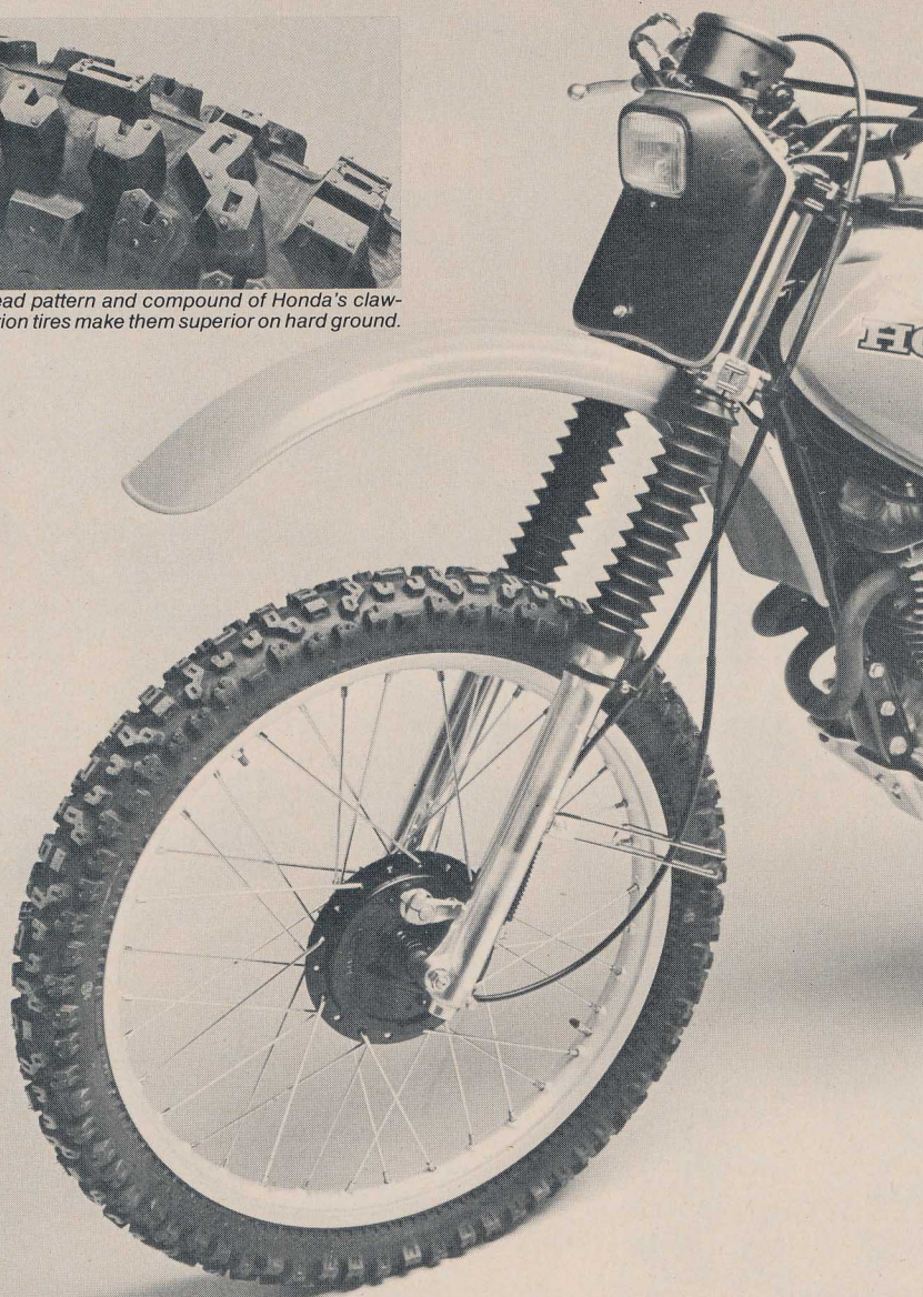
Fork with 8.8 inches of travel provides good performance for play riders; it's just adequate for competition.
