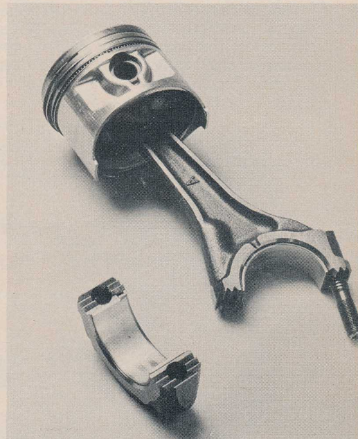
1300's rod big end parts on a bias so that rod and piston can be removed together through a cylinder bore
