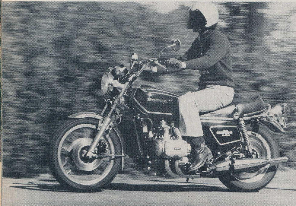
The front fork works pretty well, but the rear shock springs are still too stiff for rider-only situations.
