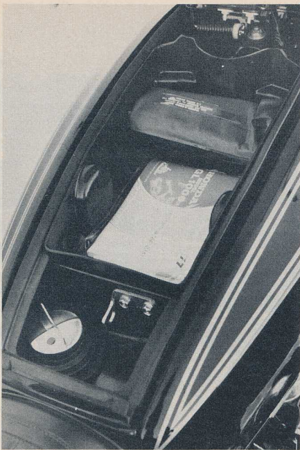
Handy storage area, gas cap and gas-catch basin are under the dummy tank's lockable top panel.
