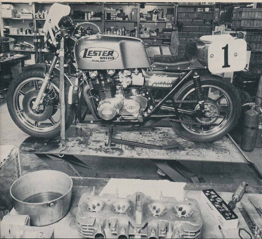
Running gear consists of Dunlop tires, S&W rear shocks, a 1976-model front fork, fiberglass tank and seat, a collector exhaust—oh, and Lester alloy wheels.
