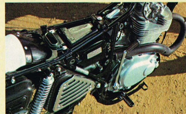
The XL-250 and 350 frames have been redesigned to provide improved steering geometry and a narrower riding position.
