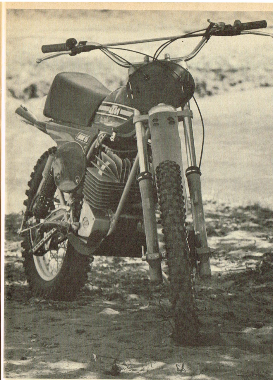
KTM did a great job of hiding the Bing carburetor. Massive cylinder fins contribute to engine's longevity. Brake pedal height is adjustable.
